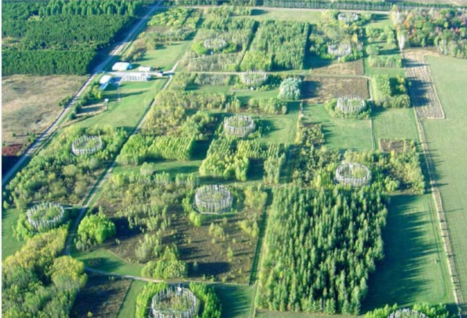
Figure 1: Free-air carbon dioxide enrichment allows experiments with controlled atmospheric concentrations of carbon dioxide to be conducted in the field and avoids potential experimental artifacts from growing plants in enclosed chambers.
